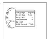
2. Press the CH+/- buttons to move the indicator to "Special", then press the VOL+ button to sub-menu.
